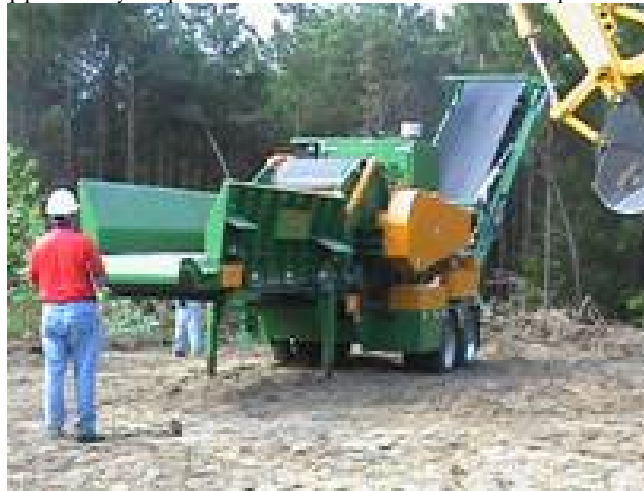
Figure 7 Precision Husky 3045 horizontal grinder at biomass harvesting site on the Talladega National Forest-Shoal Creek District
