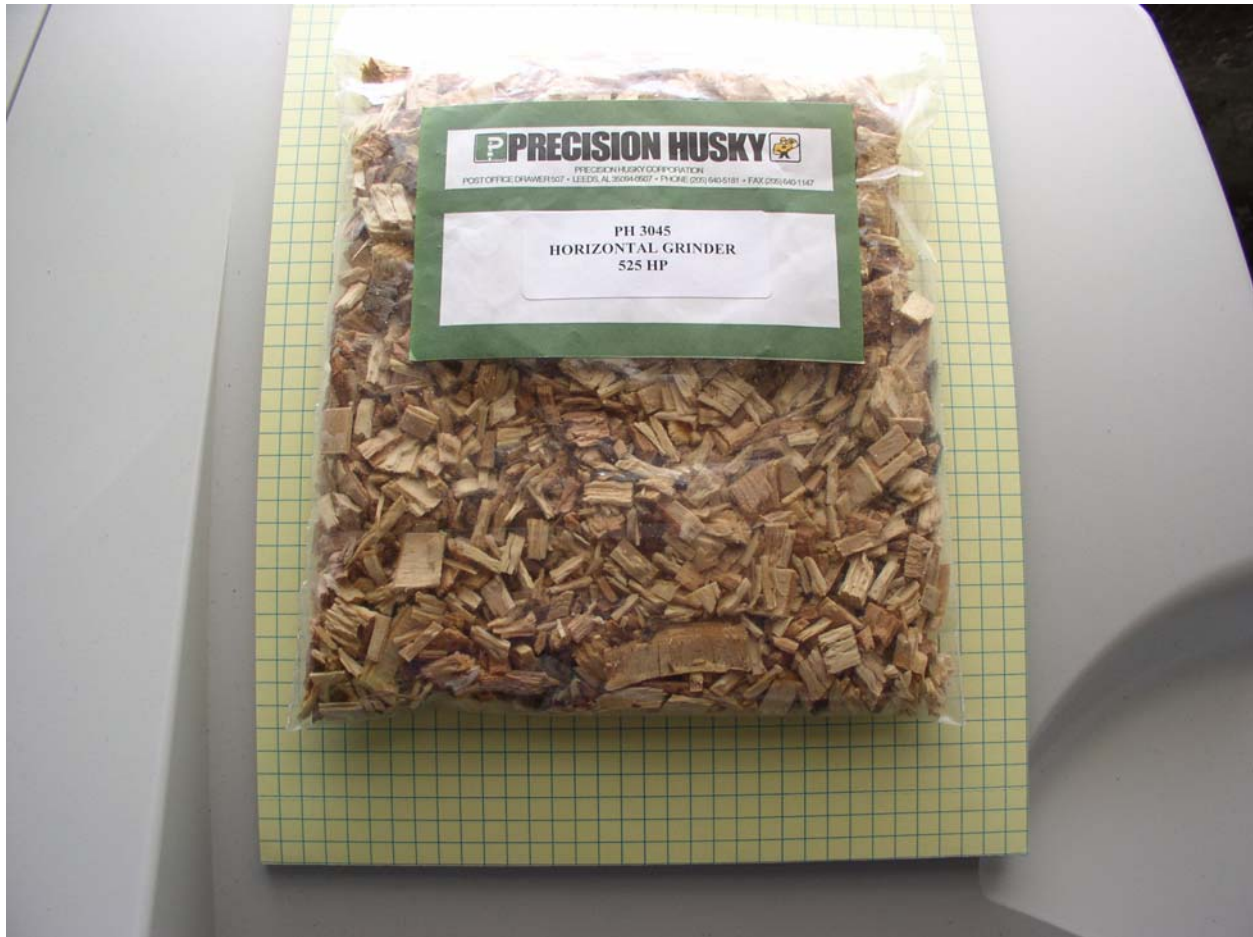
Figure 4 Wood Chip Sample Produced by PH 3045 Horizontal Grinder
